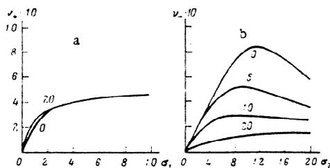
Fig. 7. Unidirectional effect of an isosteric modifier ( $\alpha$ ) on the rates of the forward (a) and reverse (b) reactions. The families  $\nu_+(\sigma_1, \alpha)$  and  $\nu_-(\sigma_2, \alpha)$  were plotted with the aid of Eqs. (32)–(33) with  $n = 4$ ,  $\kappa = 0.2$ ,  $c_\alpha = 0$ ,  $c_1 = 1$ ,  $c_2 = 10^{-4}$ ,  $a = 0.5$ ,  $L = 5 \cdot 10^4$ , and  $\sigma_2 = 0$  (a) and  $\sigma_1 = 0$  (b). The numbers on the curves are the values of  $\alpha$ .
