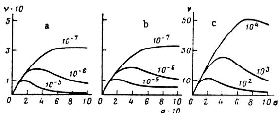
Fig. 2. Substrate inhibition of the reaction rate described by Eq. (16) for  $n = 4$  and  $a = 0$ ,  $c = 100$  (a),  $a = 4$ ,  $c = 100$  (b), and  $a = 1$ ,  $c = 0.01$  (c). The numbers on the curves are the values of  $L$ .
